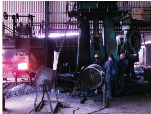
Figure 68: FO fired forging furnace
