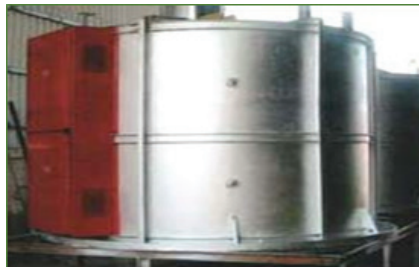
Figure 70: Bell type heat treatment furnace
