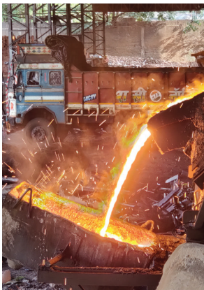
Figure 25: Tapping in progress
